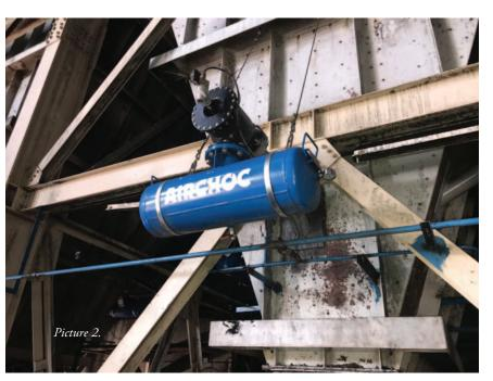
inside to prevent it from clogging, thanks to regular shots of air. This is an economical solution that uses air only when the shots are activated. With a wide range (tank capacity from four litres to 400 litres), this solution is suitable for many sectors that handle — including the coal sector.
