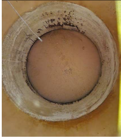
Photo 5. Before silo cleaning started. Completely bridged.
