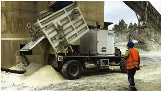
The vacuum cleaner on trailer enables the operator to carry out cleaning operations, as well as heavy pumping with a large scope of possible actions.
